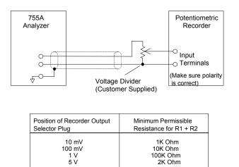
Figure 2-3. Connections for Potentiometric Recorder with Non-Standard Span
